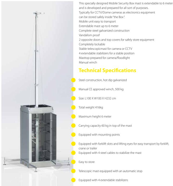
and is developed and prepared for all sort of purposes. Typically for CCTV/Dome cameras as electronics equipment can be stored safely inside "the Box". Mobile unit easy to transport Extendable mast up to 6 meter Complete steel galvanized construction Vandalism proof 2 opposite doors and top covers for safely store equipment Completely lockable Stable telescopicmast for camera or CCTV 4 extendable stabilizers for a stable position Masttop prepared for camera/floodlight Manual winch
